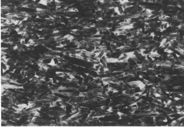
Fig. 1.1. TEM of cross-section of tape composed of oriented  $\text{CrO}_2$  particles. Courtesy of Eberhard Köester, BASF, Ludwigshaven, Germany.
